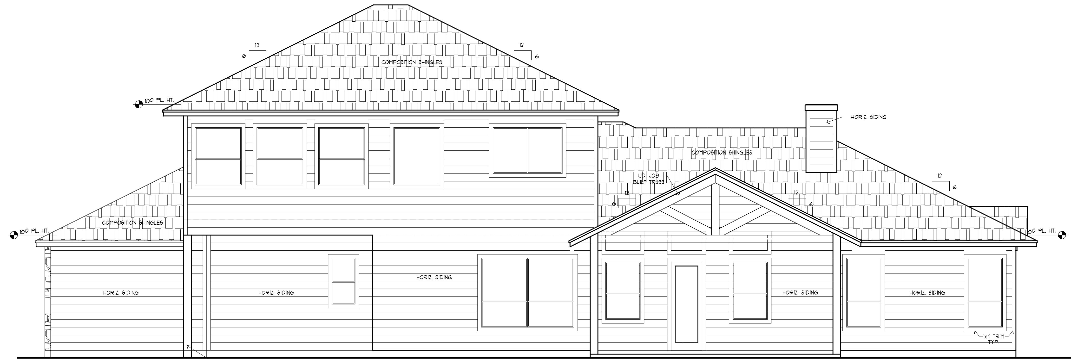
2 REAR ELEVATION SCALE: 1/4" = 1'-0"
